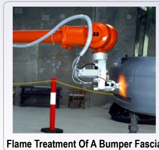
Flame Treatment Of A Bumper Fascia
